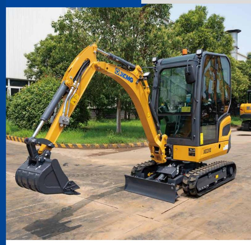
Rated Power: 11.8 kW Operating Weight: 2,050 kg Standard Bucket Capacity: 0.04 m<sup>3</sup>
